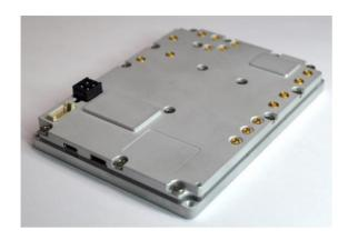
The K6 Canceller suppresses the interference a transmitter presents to a co-located receiver, even if the two radios operate with zero guard band in between them. It allows unprecedented densification and spectrum utilization in every RF environment. The solution adapts in real-time to the changing reflection environment to ensure consistent high isolation between the two radios.
