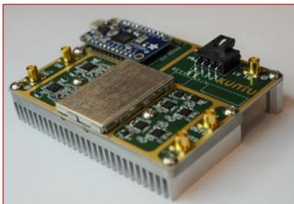
▲ Fig. 6 Kumu Networks' RFIC evaluation board.
